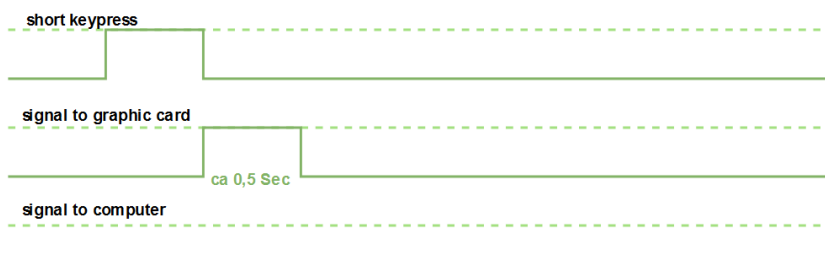
Illustration 19: Digital timing diagram - display
